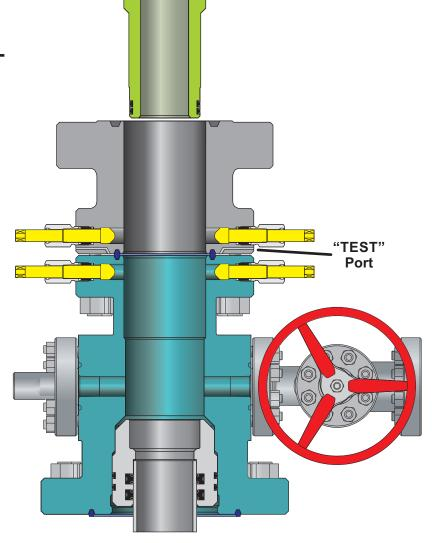
6 ☐ Completely back out ALL of the lock down pins on the Frac Adapter.
