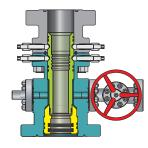
The Frac Sleeve is installed in the tubing head "in-shop", and arrives on location pre-tested.
